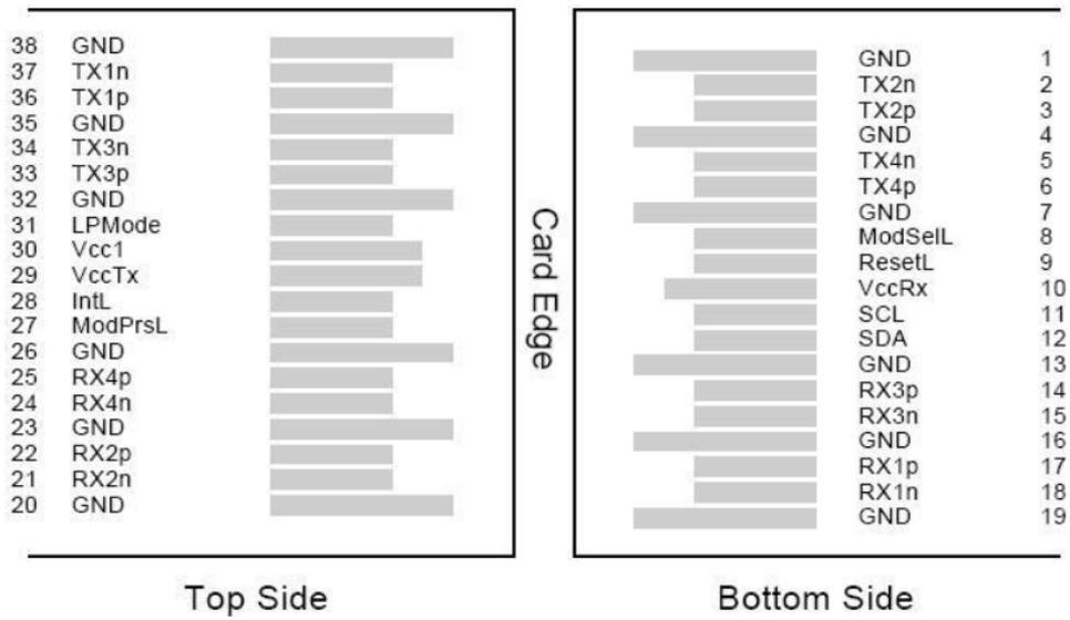
Figure 1. Host PCB QSFP+ pad assignment top view
