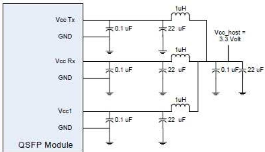
Figure 2. Recommended Host Board Power Supply Filter Network
