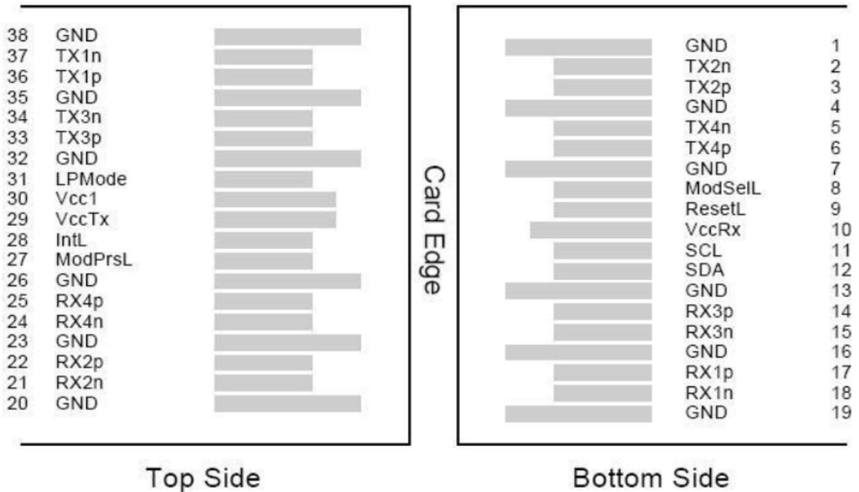
Figure 1. Host PCB QSFP28 pad assignment top view
